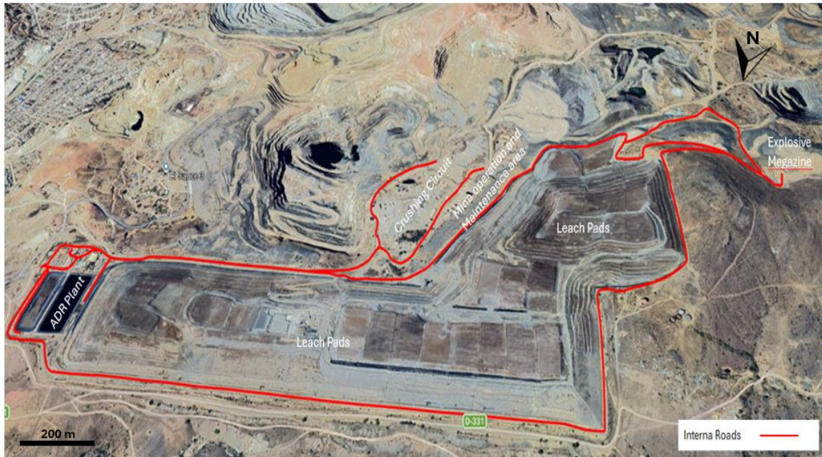
Figure 24.11 –Project Internal Site Roads Arrangement
