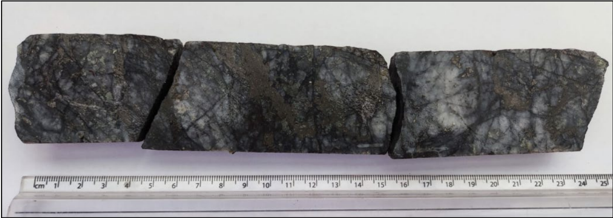
Figure 2: Split section of drill core from hole FR-DD-23-196, sample length 0.25 metre. Assay results are pending*.
