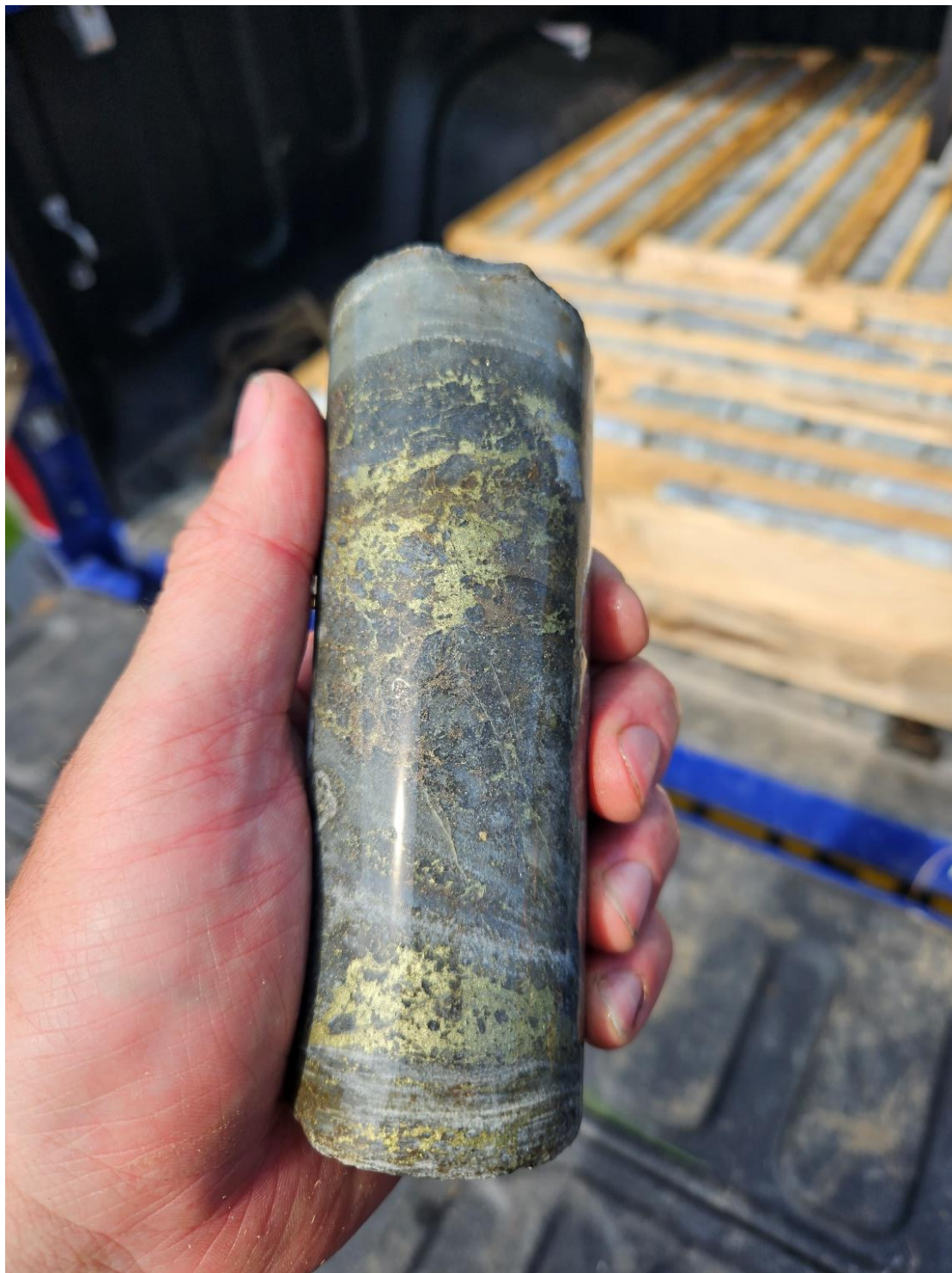
Figure 1: Section of drill core from hole 23-GL-02 showing rich chalcopyrite (a sulphide mineral that contains approximately 34% copper by weight).
