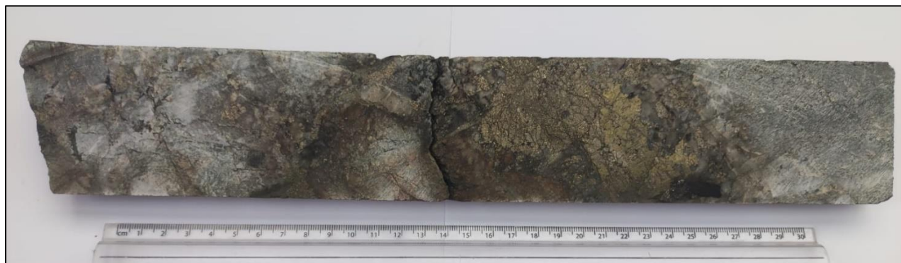
Figure 1: Part of a split section of drill core from hole FR-DD-23-UG-193 grading 72.4 g/t Au and 38 g/t Ag over a 0.36-metre core length.
