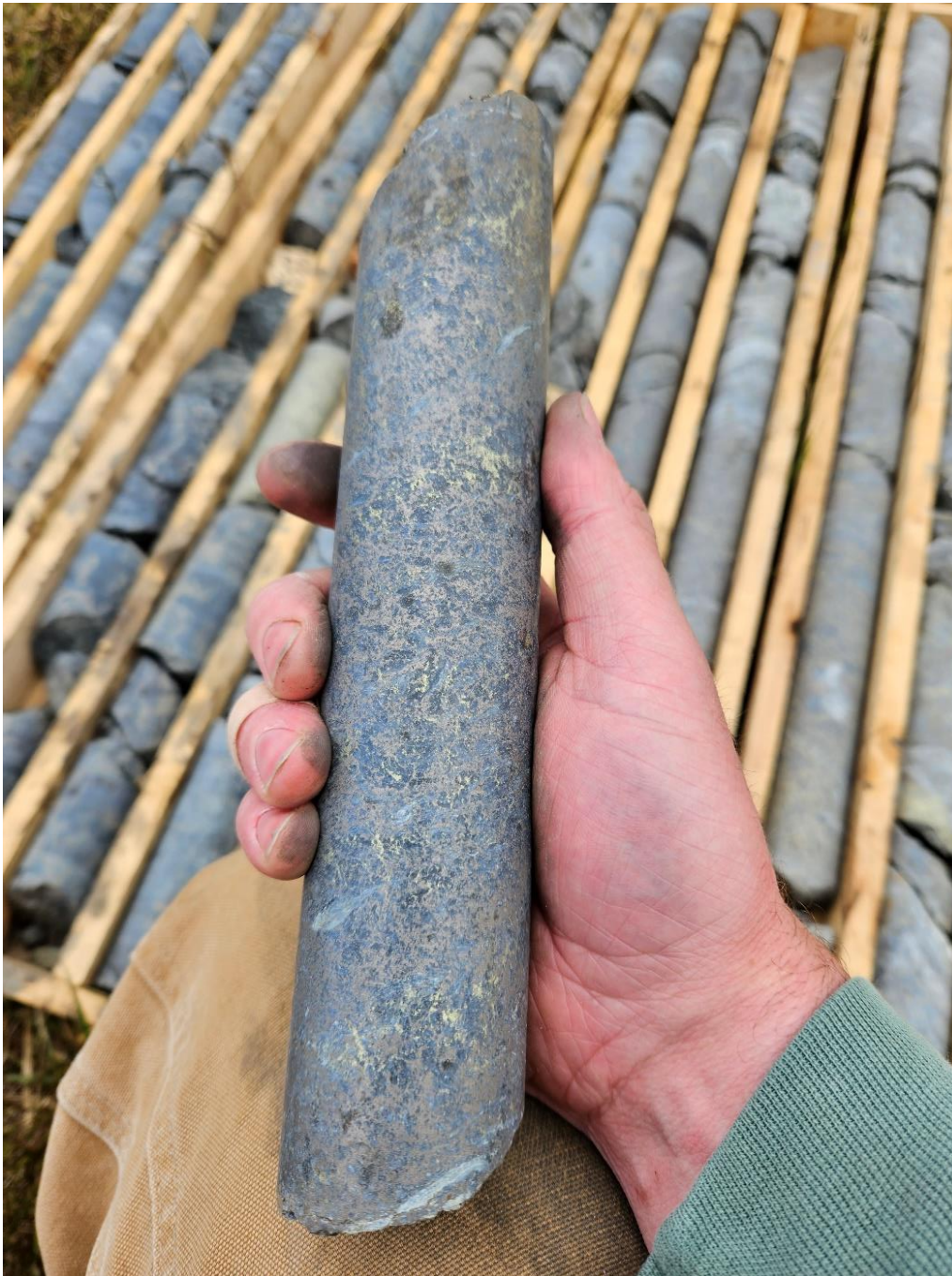
Figure 1: Part of a split section of drill core from hole 23-GL-01 showing massive sulphide.
