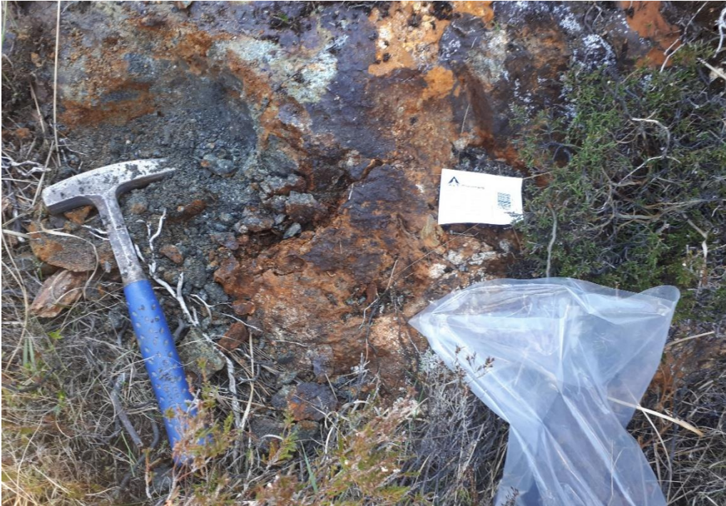
Figure 4: Second outcrop at Kerry Road deposit with visible chalcopyrite, 30 metres northwest of main outcrop, grading 2.16 g/t Au, 14 g/t Ag, 5.23% Cu and 0.30% Zn. Photo and data obtained from GreenOre.
