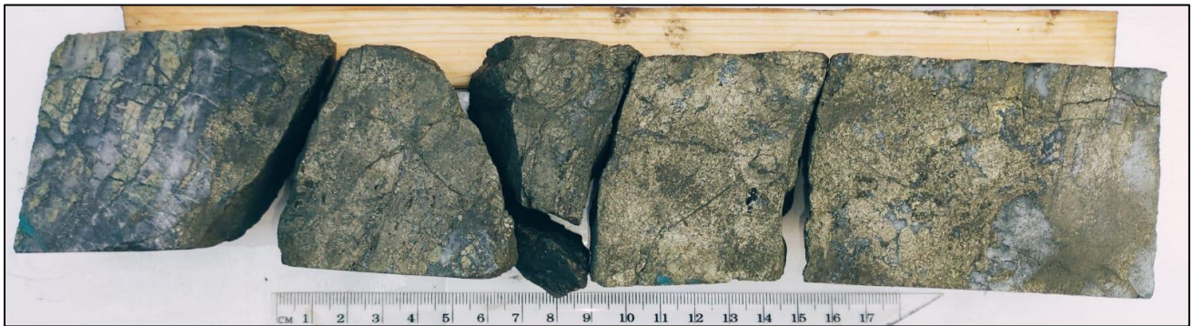
Figure 2: Split section of drill core from hole FR-DD-22-UG-183 grading 75.9 g/t Au and 90 g/t Ag over 0.26 metres.
